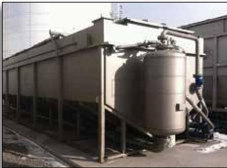
CMI's SUPERFLOT-BIOGAS™ unit, developed by Global Water & Energy, is shown here. The system is used for high-efficiency removal of anaerobic biomass from the effluent of an anaerobic treatment system.
