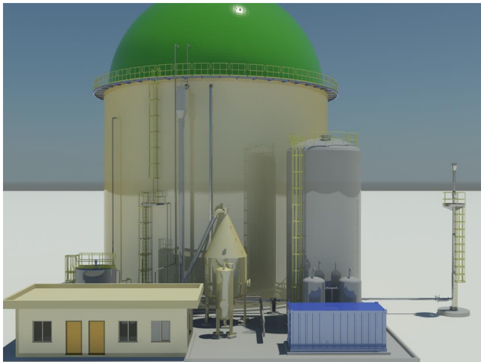
Schematic of a typical GWE anaerobic installation
