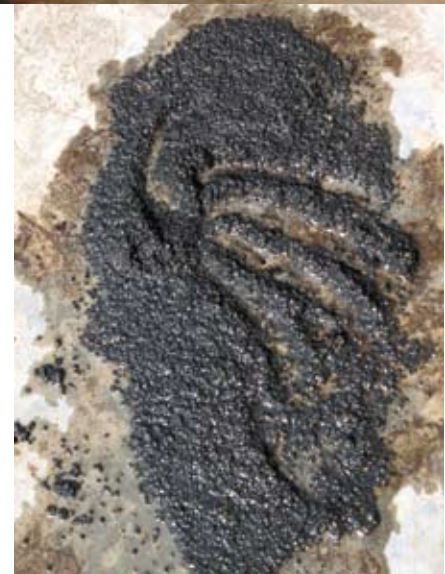
The granular sludge taken from the methane reactor. This anaerobic granular sludge is the heart of the system as it is responsible in converting the pollutants in the wastewater into biogas.
